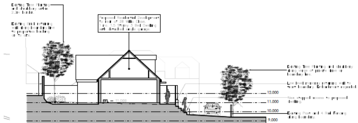
Site Proposed Site Section A-A - 1:200
